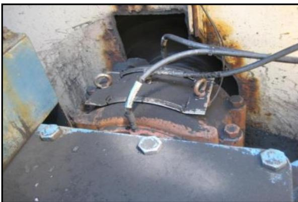
The fibre optic cable was looped across the top of the bearing housing surface and covered by a stainless-steel plate as shown in Figure 11, for both cable protection and maximising the contact surface between the fibre cable and the bearing.
