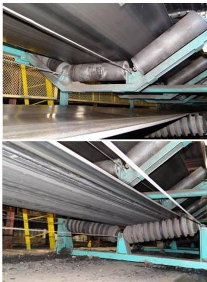
**Figure 17 Polaniec Coal Mine Carry and Return Idler Temperature Monitoring Fibre Installation**
